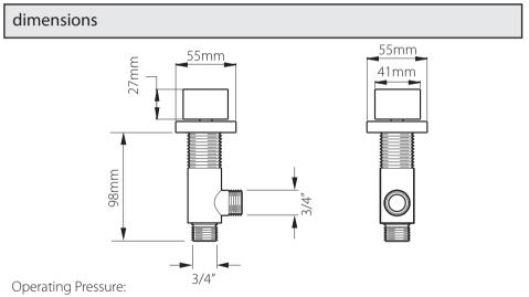
Minimum operating pressure 0.2 bar - Maximum operating pressure 5 bar
