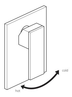
Moving the contol lever anti-clockwise will decrease the water temperature. Pull the handle out to increase the flow of water.
