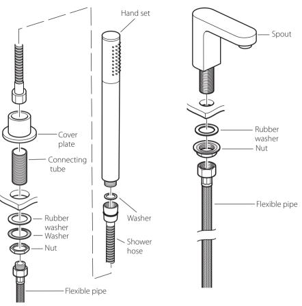
Screw the connecting tube into the cover plate and position in the hole, from the underside slide on the rubber washer, metal washer and then the nut. Tighten the nut to clamp on the cover plate.
