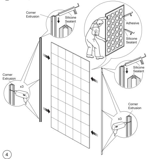
Drill 3 holes in each of the corner extrusions for the No.6 x 25 countersunk head self tapping screws.
