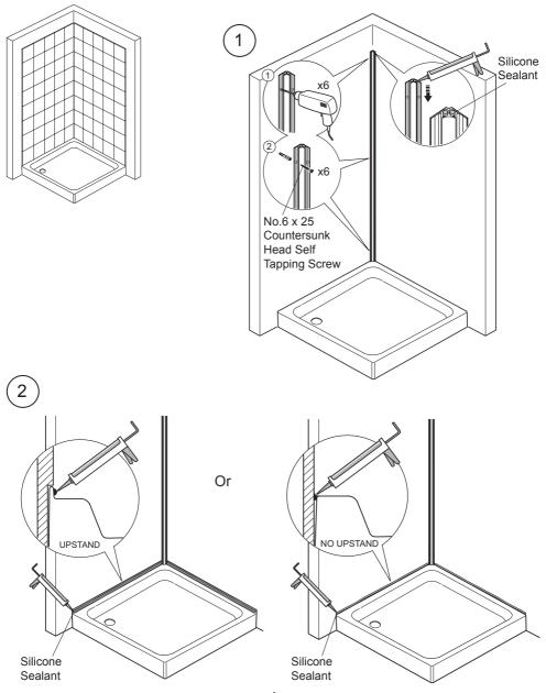
Cut any holes required for pipework. Seal the edges around the holes with silicone sealant. Apply the silicone sealant around the edge of the wall panel. Adhesive Note! The circular pattern of adhesive creates a suction effect when the flight wall is pushed flat onto the wall. Silicone Sealant 3 mm NO UPSTAND 3 mm 3 mm Spacers
