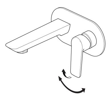
Moving the control lever anti-clockwise will decrease the water temperature.
