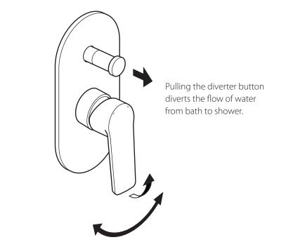
Moving the control lever anti-clockwise will decrease the water temperature. Pull the handle out to increase the flow of water.
