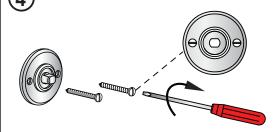
Screw in the stainless steel screws to secure the base to the wall. Please ensure that the screw heads are parallel to the floor.
