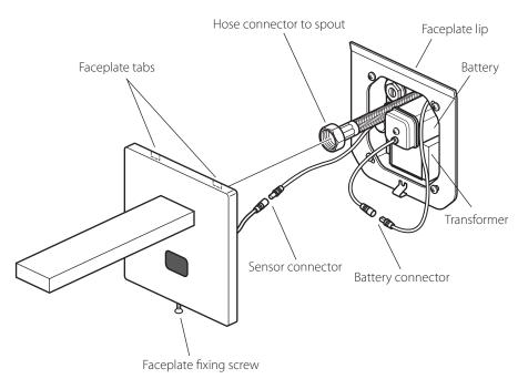
Connect the cable coming from the faceplate sensor to the valve unit.
