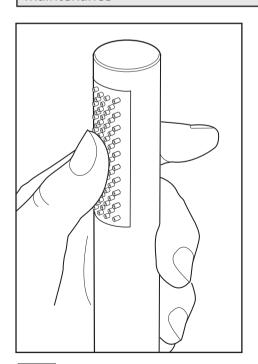
To remove any build up of limestone on the handset and showerhead, just rub your fingers lightly over the nozzles.
