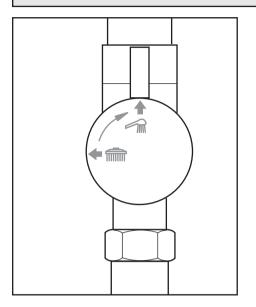
To divert the water from the handset to the riser, turn anti-clockwise.
