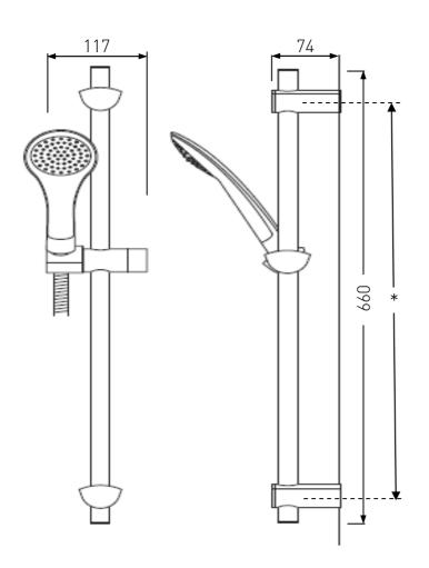
\* Note: The Riser rail wall brackets can be positioned up or down the riser rail as required. This allows any existing holes to be reused or covered by the wall brackets. The brackets can also be adjusted to sit in the middle of the tiles or in the tile joints. EV KIT02 C
