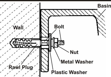
**N.B. On Some basins the sleeve on the Plastic washer wont fit through the Fixing Hole of the basin - simply remove with a hacksaw if this is the case.**
