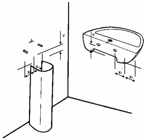
6. On the back of the basin draw a horizontal line through the centres of each fixing hole and a vertical line directly down the original centre mark on the tap ledge.
