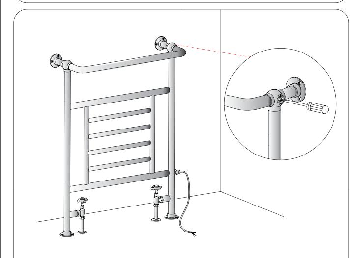
Connect to the electric supply via a fused spur. Then check for leaks. At all times follow the installation instructions supplied with the Summer Electric Heating kit. All electric work must be done by a suitably qualified person.
