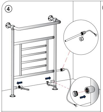
6 Connect to the electric supply via a fused spur. Then check for leaks. At all times follow the installation instructions supplied with the Summer Electric Heating kit. All electric work must be done by a suitably qualified
