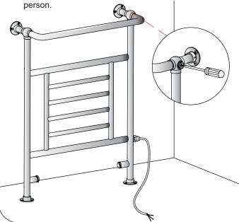
If the radiator is to be used for electric heating only ( not connected to a central heating system ), then seal the bottom inlet / outlet nipples with the blanking plugs.
