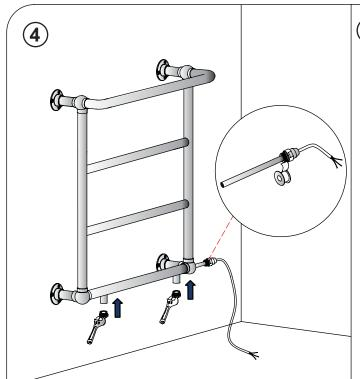
Connect to the electric supply via a fused spur. Then check for leaks. At all times follow the installation instructions supplied with the Summer Electric Heating kit. All electric work must be done by a suitably qualified
