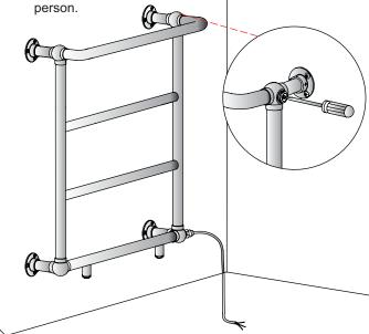
If the radiator is to be used for electric heating only ( not connected to a central heating system ), then seal the bottom inlet / outlet nipples with the blanking plugs.
