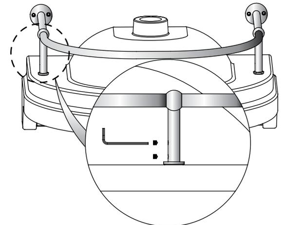
5 Mark and drill the holes in the correct position on the wall before mounting the basin
