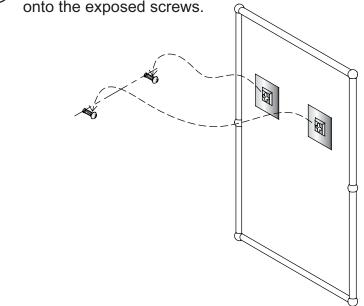
**(5)** Check that it is stable. If not please readjust the exposed length of screws .
