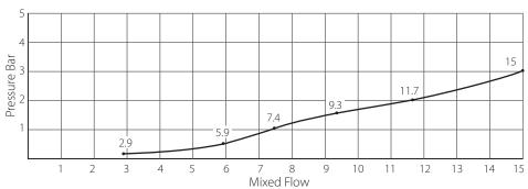
Flow rate curve is for reference only. The actual pressure drop may vary depending on system temperature and pressure.
