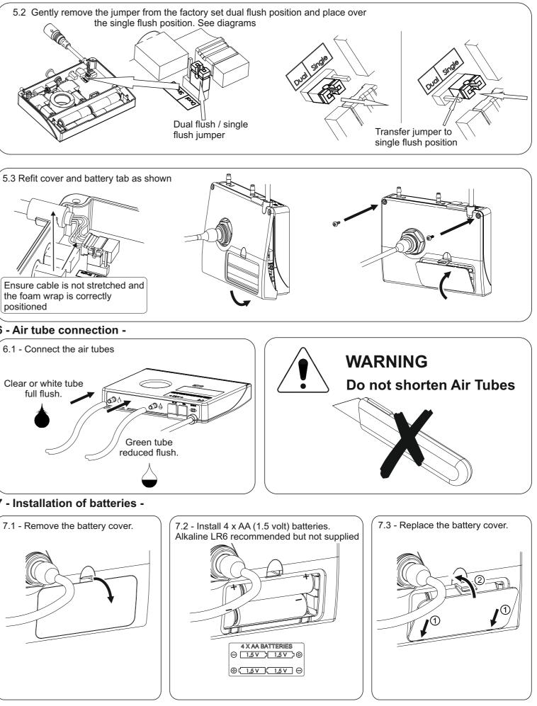
7.4 - On installation of batteries the sensor will flash red, green, blue repeatedly for 5 seconds. After this a red light will flash every 8 seconds to show the unit is active.
