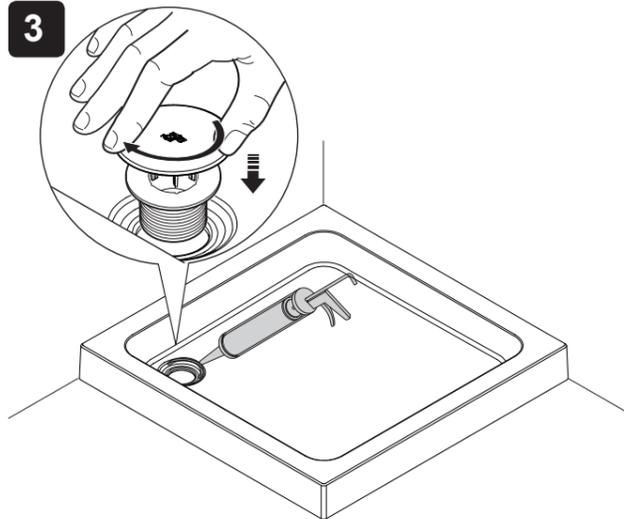
Install the waste. Hand tighten to ensure a correct seal. Install connecting pipework in accordance with Building Regulations.
