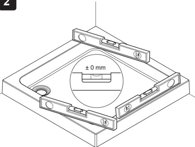
Place the shower tray on a flat surface and using a spirit level check that it is straight and flat and that the shower cubicle will sit on its surface correctly when fitted.
