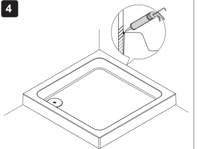
Apply silicone sealant in accordance with the manufacturer's instructions to seal the shower tray to the wall.
