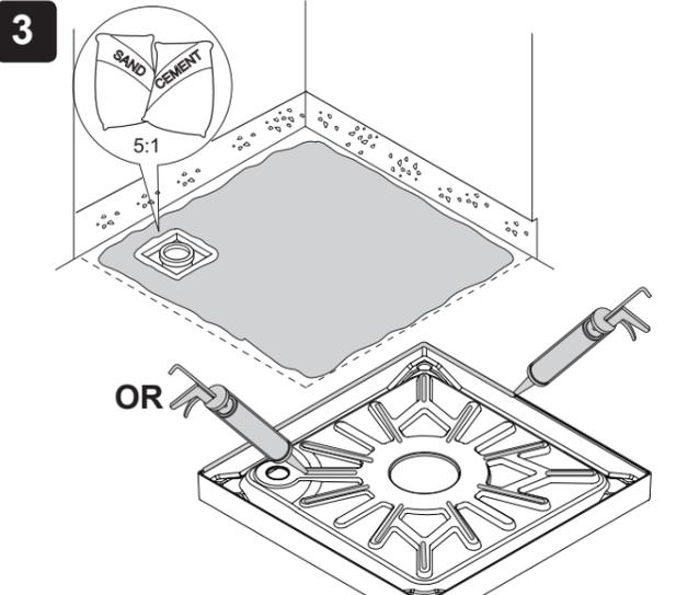
Install the shower tray on a bed of sand and cement or silicone sealant.
