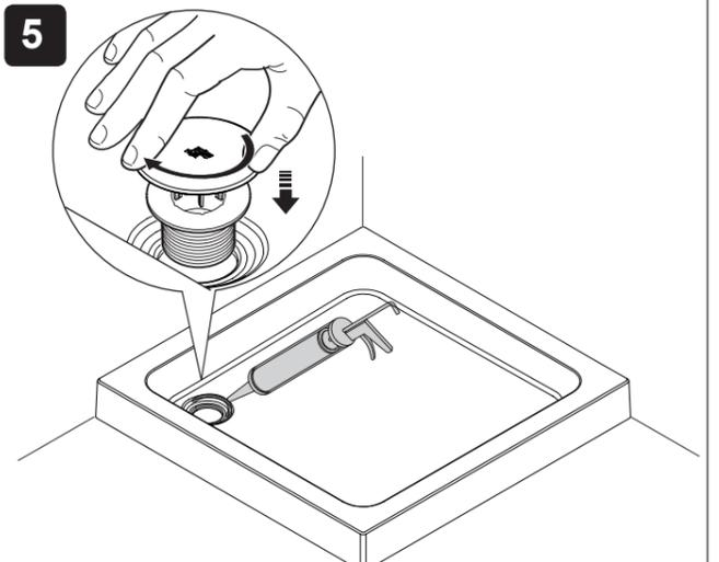
Install the waste. Hand tighten to ensure a correct seal. Install connecting pipework in accordance with Building Regulations.
