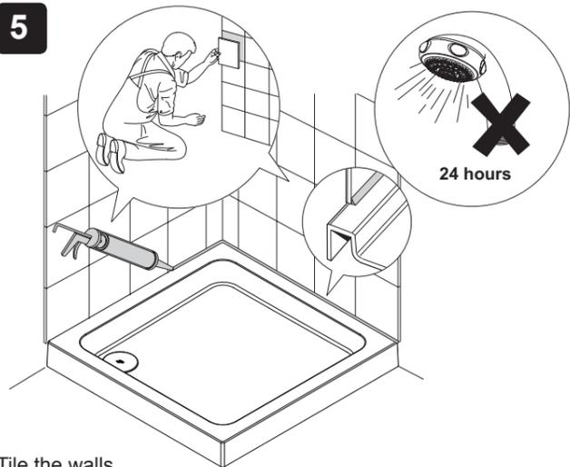
Tile the walls. Apply silicone sealant in accordance with the manufacturer's instructions to seal the shower tray to the tiled wall surface.
