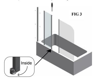
5. Ensure the bottom seal on the moving panel **A** is parallel to the top surface of the bath. Drill 3 holes through the wall profile and fixed panel using a 3mm steel drill bit. Using the Screws **2SY50** and cover caps **2SS008** and clips **2SS009**, fix the hinge upright to the wall profile in 3 places. Fig 4.
