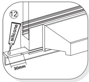
**Note:** Remove spacers in frame. Insert seal **8SSJ074** into the top and bottom profile. On both ends, pull out 30mm and put silicone on the top of the seal and reinsert.
