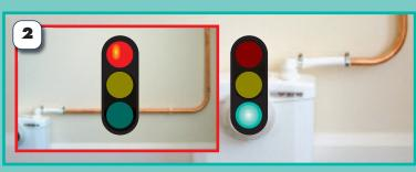
If a vertical run is needed, this should be at the start of the run (within 30cm of the unit) and from the high point there must be a minimum fall of 1:100 (see rule 1).
