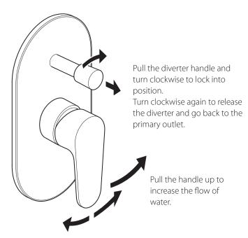
Turn the handle clockwise to increase the temperature and anti-clockwise to decrease the temperature.
