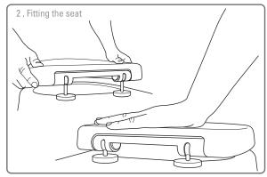
Align and insert the pins into the seat hinge sockets and firmly press down until you hear them 'click' into position.
