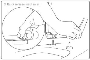
This toilet seat is designed for quick and easy removal when cleaning the toilet pan. To activate the quick release lift the lid, seat up and press the button in the centre of the hinges and lift. To replace the seat align the sockets with the pins and firmly press into position.
