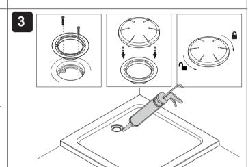
Install the waste. Tighten to ensure a correct seal. Do not overtighten. Install the connecting pipework in accordance with Building Regulations.
