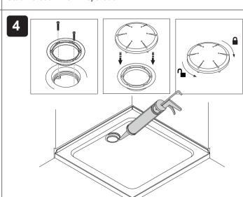
Install the waste. Tighten to ensure a correct seal. Do not overtighten. Install connecting pipework in accordance with Building Regulations.
