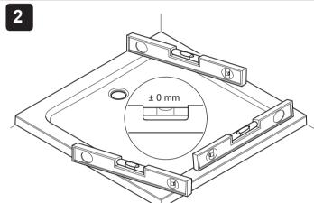
Place the shower tray on a flat surface and using a spirit level check that it is straight and flat and that the shower cubicle will sit on its surface correctly when fitted.
