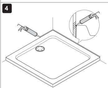
Apply silicone sealant in accordance with the manufacturer's instructions to seal the shower tray to the wall.
