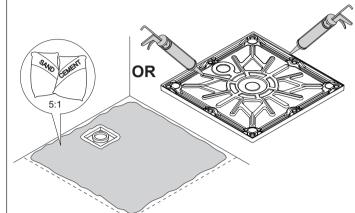
Install the shower tray on a bed of sand and cement or silicone sealant.
