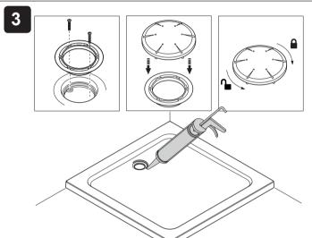
Install the waste. Tighten to ensure a correct seal. Install connecting pipework in accordance with Building Regulations.
