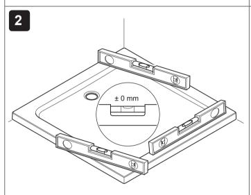
Place the shower tray on a flat surface and using a spirit level check that it is straight and flat and that the shower cubicle will sit on its surface correctly when fitted.
