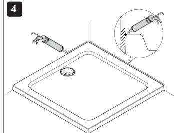
Apply silicone sealant in accordance with the manufacturer's instructions to seal the shower tray to the wall.
