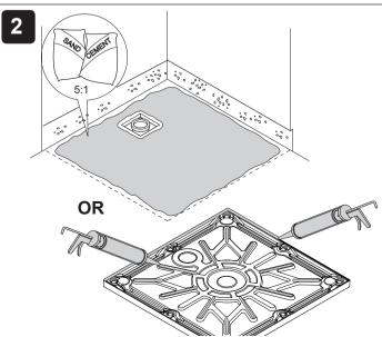
Install the shower tray on a bed of sand and cement or silicone
