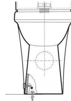
4. Using the nylon spacer, screw through the side of the pan into the L Shaped Bracket to secure the pan in place.
