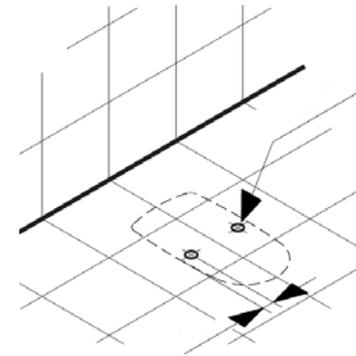
2. From the outline of the Pan mark inside the thickness of the pottery to position the L Shape Bracket.
