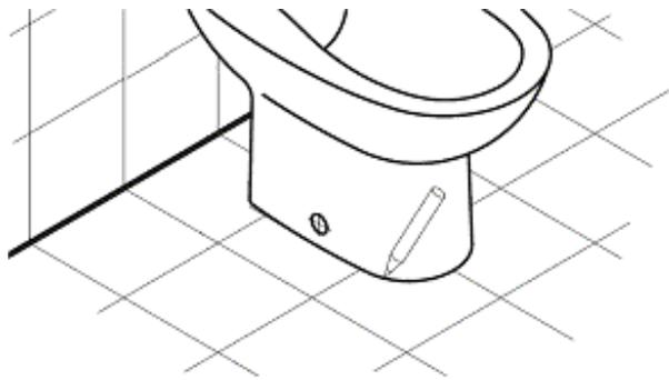
1. Position Pan in desired location. On the outside of the Pan mark the location of the fixing hole.
