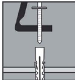
3. Check plug dimension and use corresponding bit size to drill as required. Fix L Bracket to floor.
