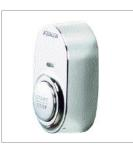
To release the button, insert a small flat bladed screw driver into the small slot at the bottom of the button assembly to release the locking clip, taking care to avoid damaging the plated surface. Carefully lift the button out and up off the back plate top locating peg.
