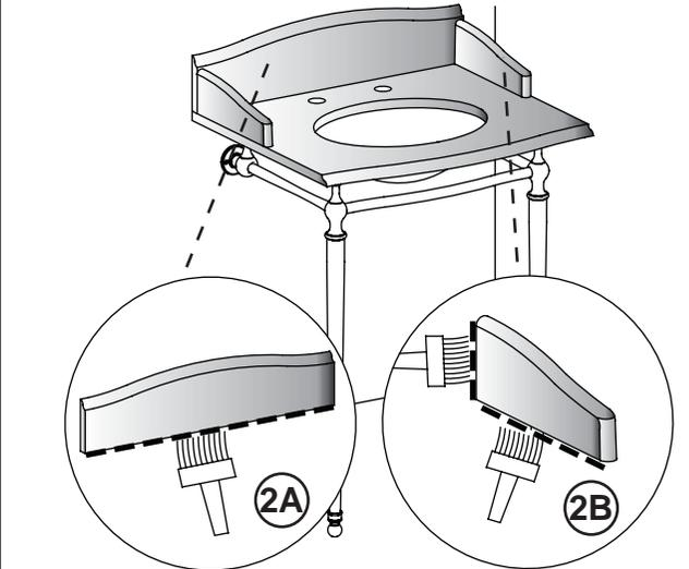
**1** Spread the AB glue on the top surface of the basin stand. Position the basin and apply gentle pressure with the base of your hand, final level the basin.
