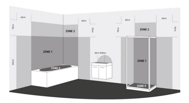
The diagram above is supplied as a guide to Bathroom Zones as referred to in IP ratings of the over mirror lamps and electric heating elements. Please refer to the latest edition of BS 7671:2008(2011) to ensure conformity.
