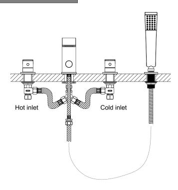
Connect the tee connector and the hot/cold control valves using braided hoses. Connect one end of the shower hose to the flexible tail of spout assembly and the other end to the shower, ensuring a washer is in.
