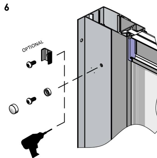
WHEN THE FRAME IS READY TO BE FIXED, DRILL THROUGH THE HOLES IN THE WALL PROFILE WITH A 3mm DRILL. (MAKE SURE YOU ONLY DRILL THROUGH ONE WALL THICKNESS) THEN FIX THE FRAME WITH ITEMS 23, 25\* & 26\*.
