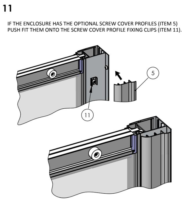
IF THE ENCLOSURE HAS THE OPTIONAL SCREW COVER PROFILES (ITEM 5) PUSH FIT THEM ONTO THE SCREW COVER PROFILE FIXING CLIPS (ITEM 11).
