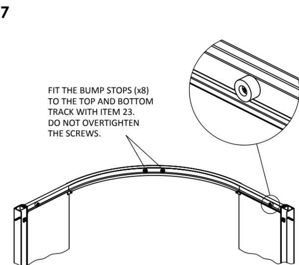
FIT THE BUMP STOPS (x8) TO THE TOP AND BOTTOM TRACK WITH ITEM 23. DO NOT OVERTIGHTEN THE SCREWS.
