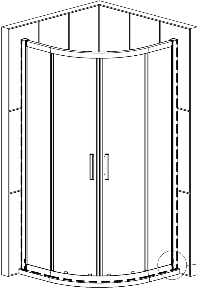
SILICONE THE PLASTIC MOULDING WITH AS SMALL A BEAD AS POSSIBLE.
