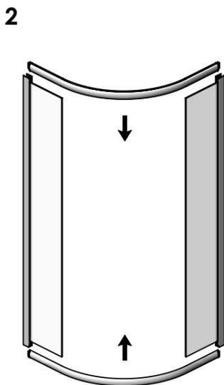
SLIDE THE TRACKS ONTO THE FIXED PANEL SUB ASSEMBLY UNTIL FLUSH WITH THE VERTICAL PROFILES.
