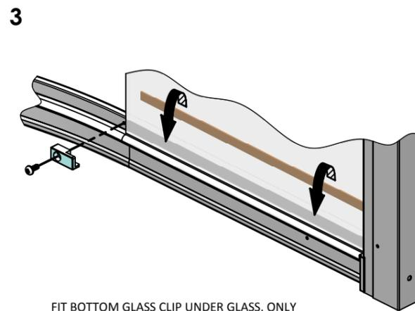
FIT BOTTOM GLASS CLIP UNDER GLASS. ONLY TIGHTEN SCREW PART WAY. FIT GLASS BOTTOM SEAL (ITEM 10) BETWEEN GLASS AND PROFILE. FIT TOP GLASS CLIP AND TIGHTEN ALL SCREWS.
