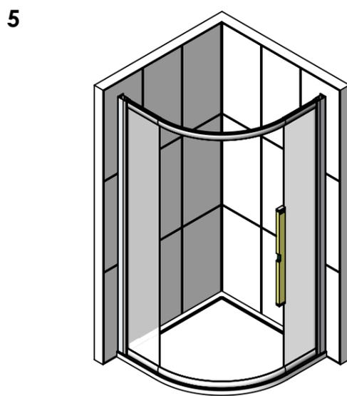
FIT THE FRAME INTO THE WALL PROFILES. ADJUSTING UNTIL THERE IS AN EVEN GAP BETWEEN THE FRONT EDGE OF THE TRAY AND BOTTOM TRACK (12mm). THERE SHOULD ALSO BE AN EQUAL AMOUNT OF FRAME IN EACH WALL PROFILE. ENSURE THE FRAME IS TRUE ON BOTH SIDES BEFORE IT IS FIXED IN PLACE.
