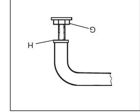
cradles. bushed ends (H) of the adjustable feet into the adjustable feet. Screw the 3. Screw nuts (G) onto the
