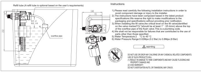
I. Work Preparation: Remove the inoperative tank fittings and carefully clean the water cistern/tank. Make sure all debris has been removed prior to installing new tank fitting.
