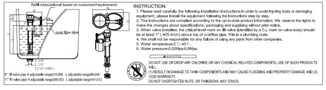
I Preparation Please remove the worn out fittings and clean your tank when you just install a new one, there might be lots of impurities in your tank, so clean your tank should be the first thing you do. II Water level adjustment
