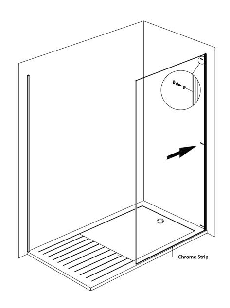
5. Ease the glass panel into the wall channel ensuring the chrome strip is at the bottom of the screen and the 'Shower Shield' is on the inside face.
