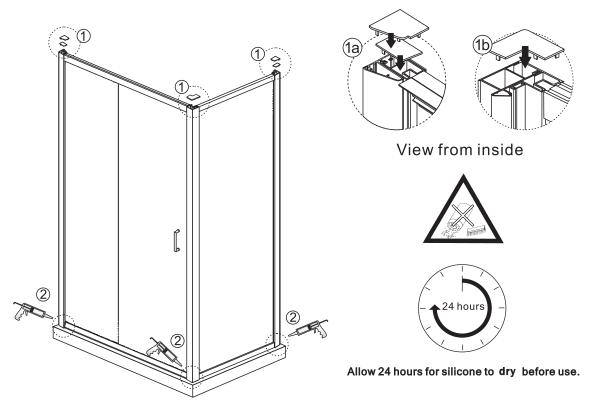
A High Grade Silicone Sealant Should Be Used and Applied Externally As And Where Required Between the Glass and Aluminium Frame and Between the Aluminium Frame and the Tiled Walls/Shower Tray
