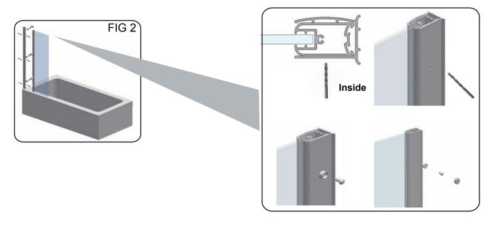
Insert the glass bracket S033C onto the long side of the rail and position towards the end of the glass panel. Insert the wall bracket S035C onto both ends of the rail. Level the rail and mark the fixing points to the wall. NOTE: Cut rail to size if required. DO NOT CUT TOO SHORT.
