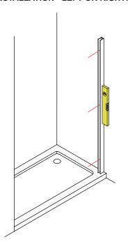
Remove the wall channel from the glass panel frame. Place the wall channel in position on the tray (10 - 15mm in from the outer edge of the tray), use a spirit level to ensure it is vertical and mark all 3 fixing holes onto the wall.
