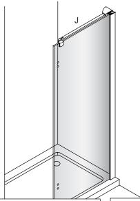
! Please note the grub screws within part (H) and part (N) need to be loosened so that the supporting bar (J) can be inserted.
