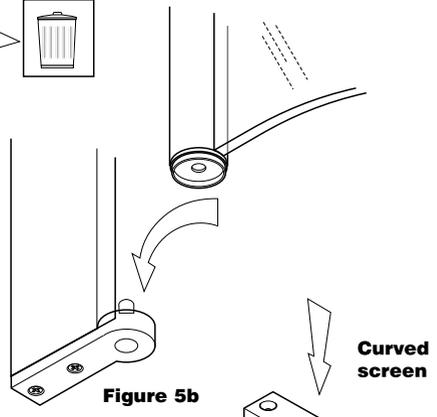
Push end casting into place on screen, Fig. 5c.
