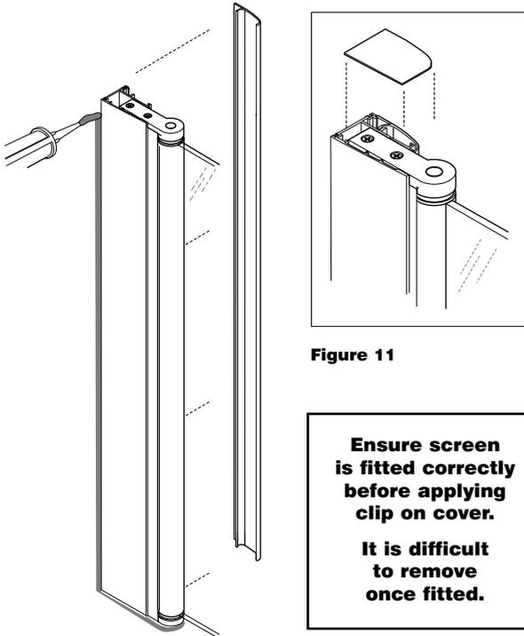
**Ensure screen is fitted correctly before applying clip on cover.**
