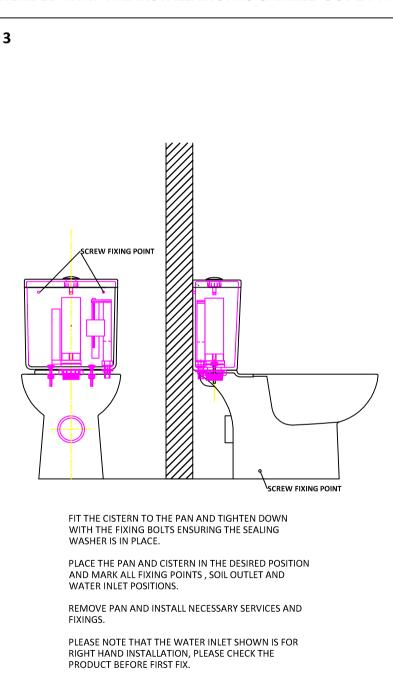
PLACE THE UNIT BACK INTO POSITION, CONNECT WATER INLET AND THE SOIL OUTLET THEN SECURE FIRMLY USING THE FIXING POINTS.
