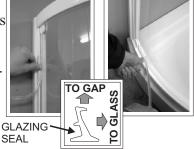
CHECK HANDING OF SLIDING DOOR- Stand door upright so that the lever patch fittings are at the bottom and the outside face of door is facing you. If the door handle is on the correct side to suit your installation, proceed to next stage.
