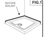
Once the walls have been tiled but **before** the enclosure is installed, the tiles **must** be silicone sealed to the tray all of the way around in one continuous bead.
