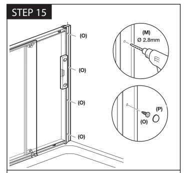
Drill both the side panel compensator and door to the wall profiles using the 2.8mm diameter drill bit (M) drill through the compensator holes into the wall profile.
