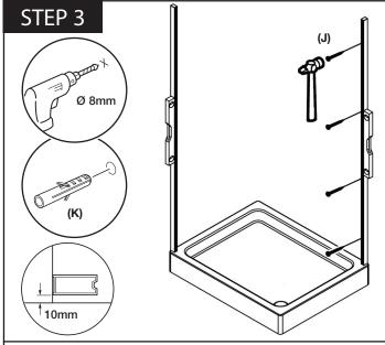
Position the wall channels onto the tray and against the wall, ensure the wall channels are perfectly vertical and **10mm** from the front and side edge of the tray. Mark off the hole positions using the centre punch (J).
