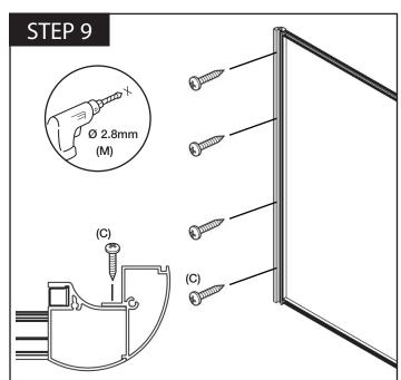
With the corner post in position drill through the holes into the compensator profile use the 2.8mm diameter drill bit (M). Screw the corner post to the compensator profile using four 13mm screws (C) as shown above.
