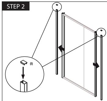
Remove the wall profiles from the compensator profile as supplied with the door unit.
