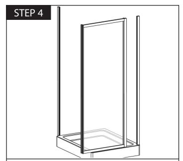
With the wall profiles fitted slide the side panel onto the tray and push on to the wall profile (push the unit back to the wall). Ensure not to scratch the tray when pushing the side panel on.
