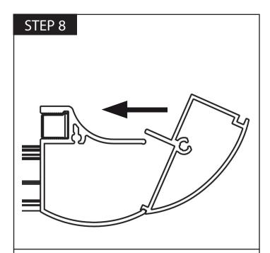
Attach the corner post to the compensator profile. Push the corner post on to the notch and rotate around ensuring the profiles stay together as shown above.
