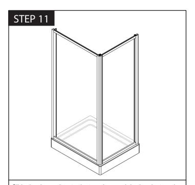
Slide the door unit onto the tray then push both units together on the tray ensuring all the profiles align.
