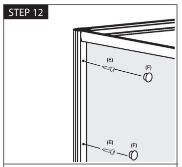
Screw the side panel to the corner post using the supplied 13  $\times$  4.2mm screws (E) and push fit the cover caps (F).
