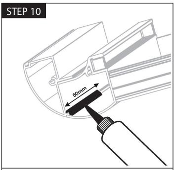
Tilt the door unit to enable access to the bottom of the corner post and compensator profile, silicone across the join covering a distance of **50mm** vertically as shown above.
