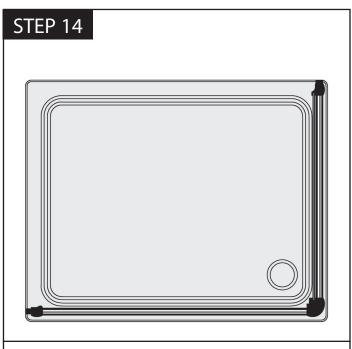
Align the unit to the tray by sliding the unit within the adjustment of the wall profile.
