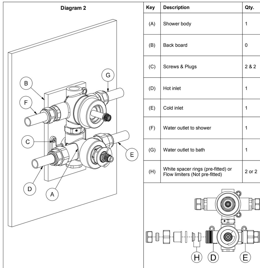
2. Fix inlet and outlet pipes securely to the wall using appropriate fixings. Inlet pipes should finish at the same height and be spaced as required.
