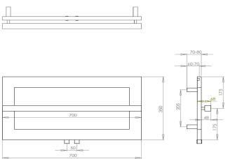
Screw 4x inserts (3) onto the nuts welded on the back of the radiator slide 4 x brackets (2) onto inserts and secur with grub screws (4).
