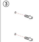
Insert the rawl plugs into the drilled holes.
