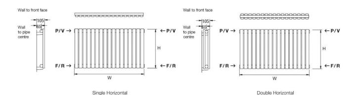
MaterialsMild SteelConnections½ Flow and returnTest pressure8 BarTesting authorityEN442Max operation pressure6 BarMax working temperature95c
