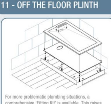
comprehensive 'Fitting Kit' is available. This raises the tray off of the floor to provide a simpler plumbing solution. For further details, see your retailer or installer.
