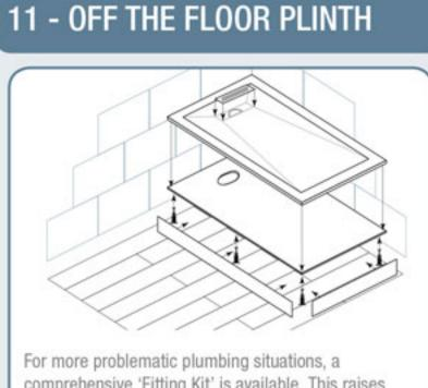
comprehensive 'Fitting Kit' is available. This raises the tray off of the floor to provide a simpler plumbing solution. For further details, see your retailer or installer.
