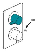
Turning the flow control handle in the direction of the arrow (anti-clockwise) increases the flow of water
