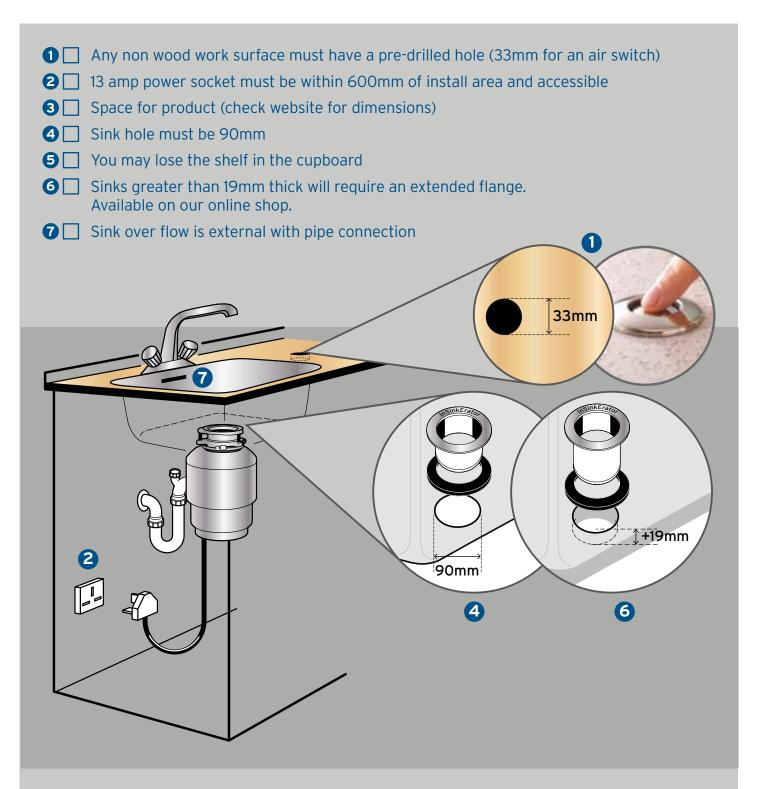
The appliance will be connected to existing services only. Should a hole not be pre-drilled in any work surface other than wood, installation will not be possible. If the criteria above has not been met on the arrival of the service agent, the customer will have to pay a call out charge of £65 to the service agent.
