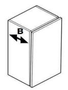
**B** - Lateral Loosen screw 'B'. Adjust door and re-tighten screw.
