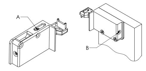
You may need to increase the length of the hook's protrusion. To do so turn screw 'B' anti-clockwise.
